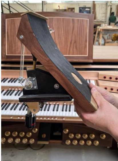
Expression pedal, with hydraulic system to adjust the force required
