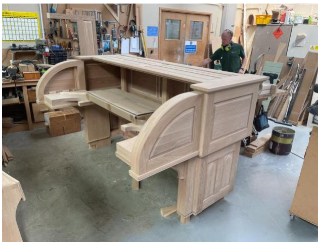
Console in construction for the American organ-builder Marshall and Ogletree
