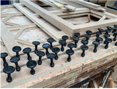
Ebony stop knobs, after turning
