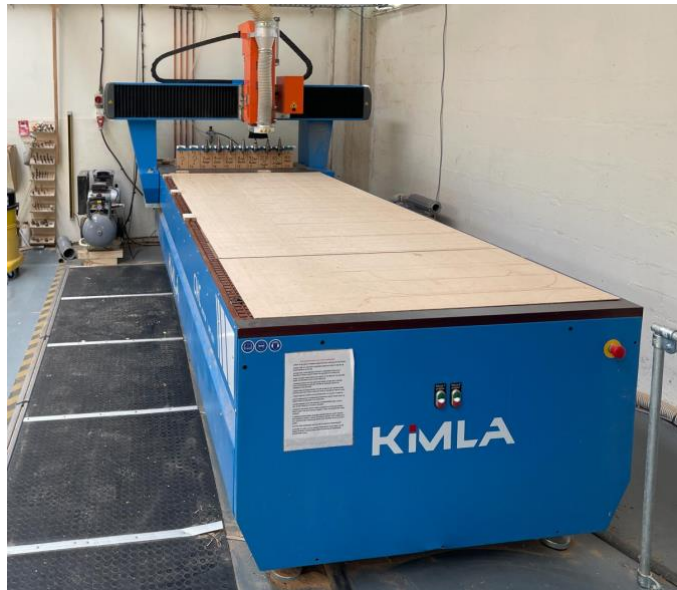
Computer controlled machine, cuts boards up to 10x4 feet
